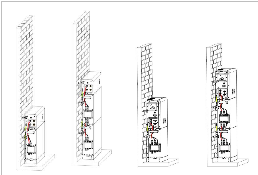
Figure. 4.1.2-3 Installation diagram of different battery quantities
